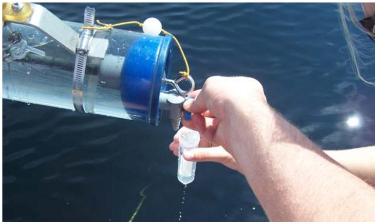
An intern pours off water from a deep water grab to be analyzed later for phosphorus concentration.
