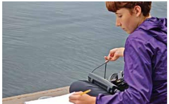
Summer 2014 intern Danae Winkler tests for dissolved oxygen and water temperature.
